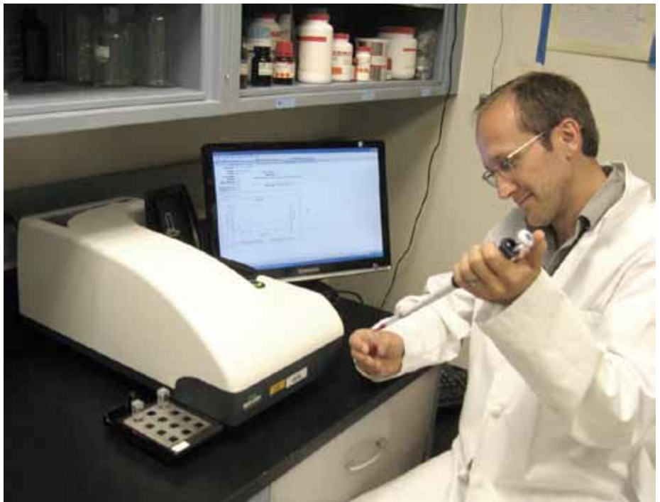
Dr. Conrad Stoldt of the University of Colorado-Boulder prepares a silicon nanocrystal sample for size analysis.
