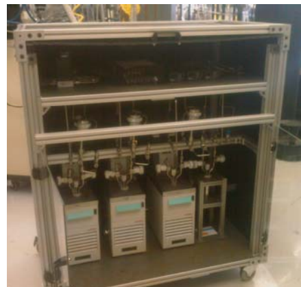
Figure 2: Photograph showing our home-built, MOCVD precursor delivery system.
